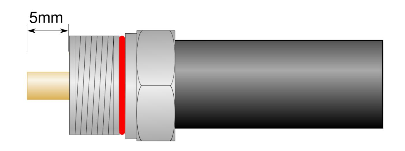
With two spanners, hold the connector body stationary and tighten the locking nut
