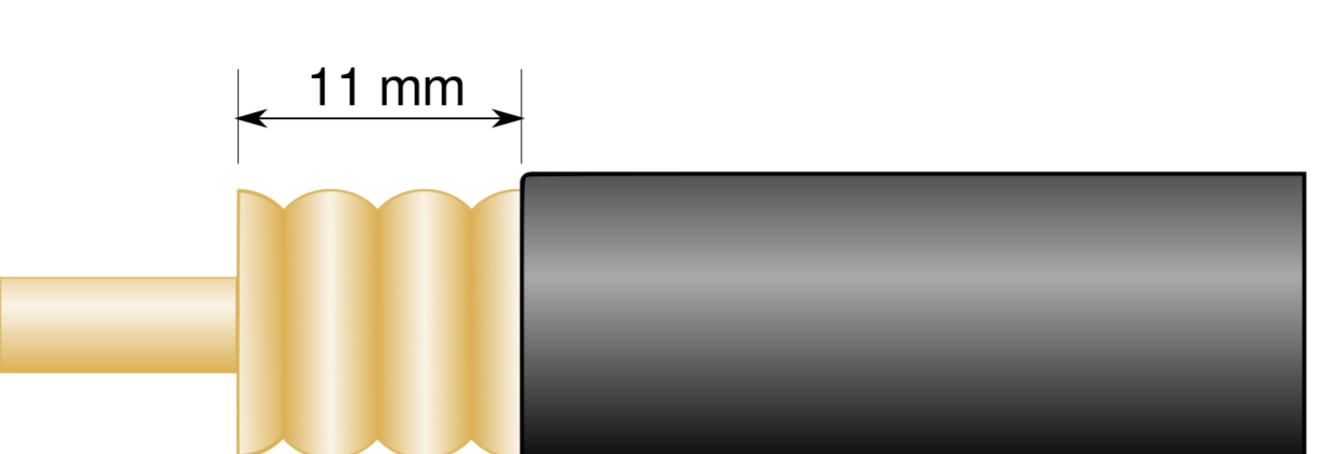
Firmly push the locking nut onto the cable, ensuring that the finger stock is seated in a valley of the cable screen
