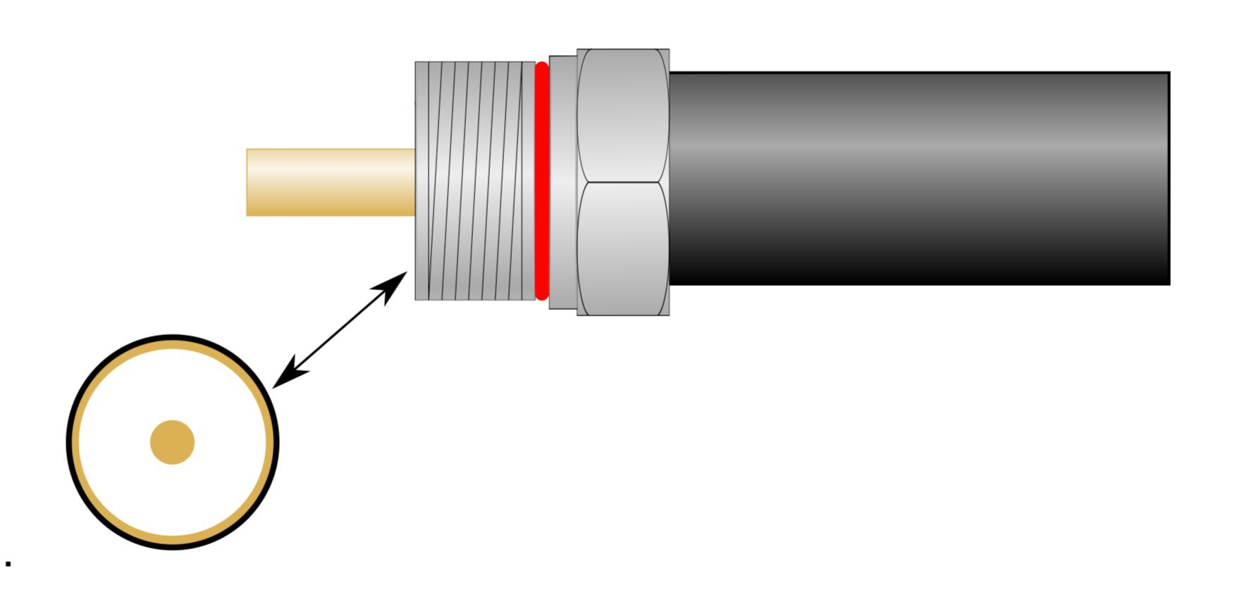
Cut the centre condutor so that 5mm is protruding from the dielectric. Ensure the end of the centre conductor is flat and clean of and debris or dielectric material
